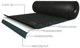
Upper coating: TPO-plastomer modified bitumen Composite reinforcement (180 g/m2) of polyester and glass fibre Uncercoating: SBS-elastomer modified bitumen
